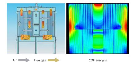
Danstoker air preheater (APH) comes with a non-corrosive design, with a hybrid cross and counter flow design that has been validated with extensive CDF analysis.
