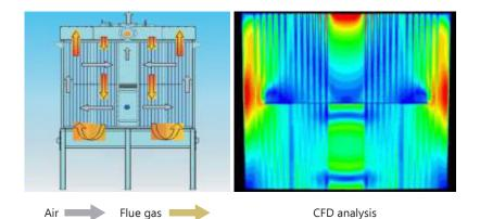
Danstoker air preheater (APH) comes with a non-corrosive design, with a hybrid cross and counter flow design that has been validated with extensive CFD analysis.
