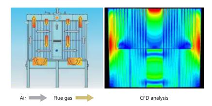
Danstoker air preheater (APH) comes with a non-corrosive design, with a hybrid cross and counter flow design that has been validated with extensive CDF analysis.
