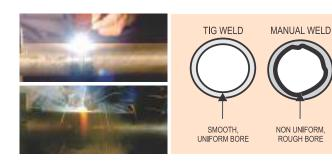
Fully automated tube to tube TIG Welding Machine enables smooth inform bore.
