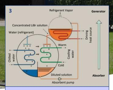
As Lithium Bromide becomes dilute it loses its capacity to absorb water vapor. It thus needs to be reconcentrated using a heat source.
