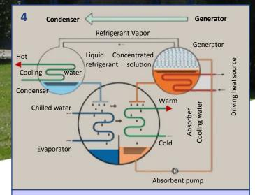
This heat causes the solution to release the absorbed refrigerant in form of vapor. This vapor is cooled in a separate chamber to become liquid refrigerant. The concentrated LiBr is sprayed back in the absorber.
