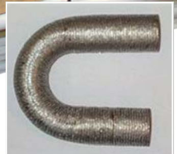
Tube with Inconel cladding and then cold bent
